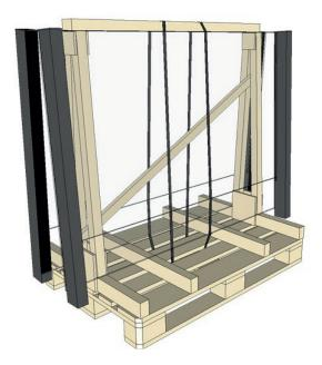
Each section is individually secured on the packaging to prevent falling during unloading.
