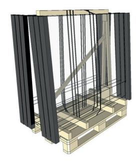
Loosen the straps gradually as sections are installed. Each package can hold up to 6 sections.
